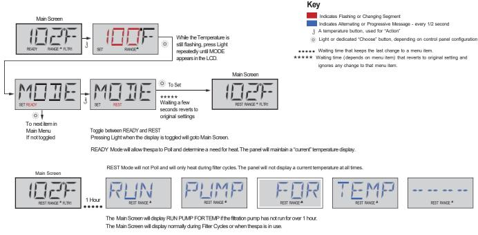
If the filtration pump has been off for an hour or more, when any function button, EXCEPT Light, is pressed on the panel, the pump used in conjuncton with the heater will run so that temperature can be sensed and displayed
