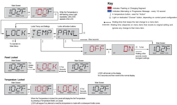
Adjustable settings in the menus are also locked. Other function buttons will operate normally.
