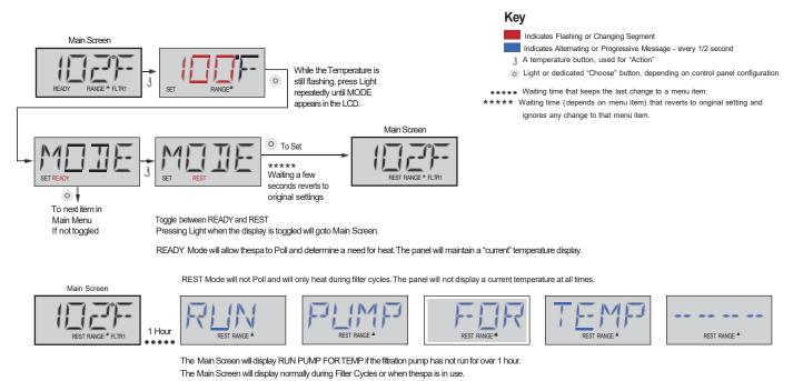
If the filtration pump has been off for an hour or more, when any function button, EXCEPT Light, is pressed on the panel,
